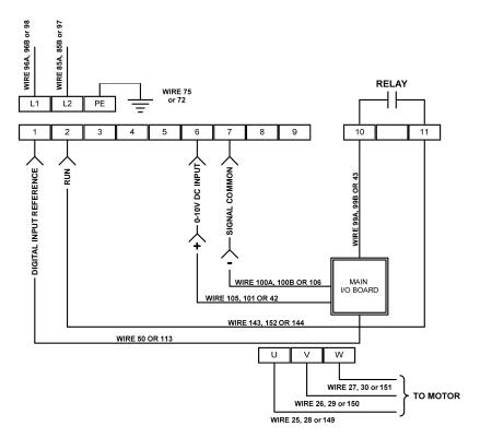
INVERTEK E3 INVERTER CONNECTIONS PS360G OR PS360GWB, 3-INVERTER
